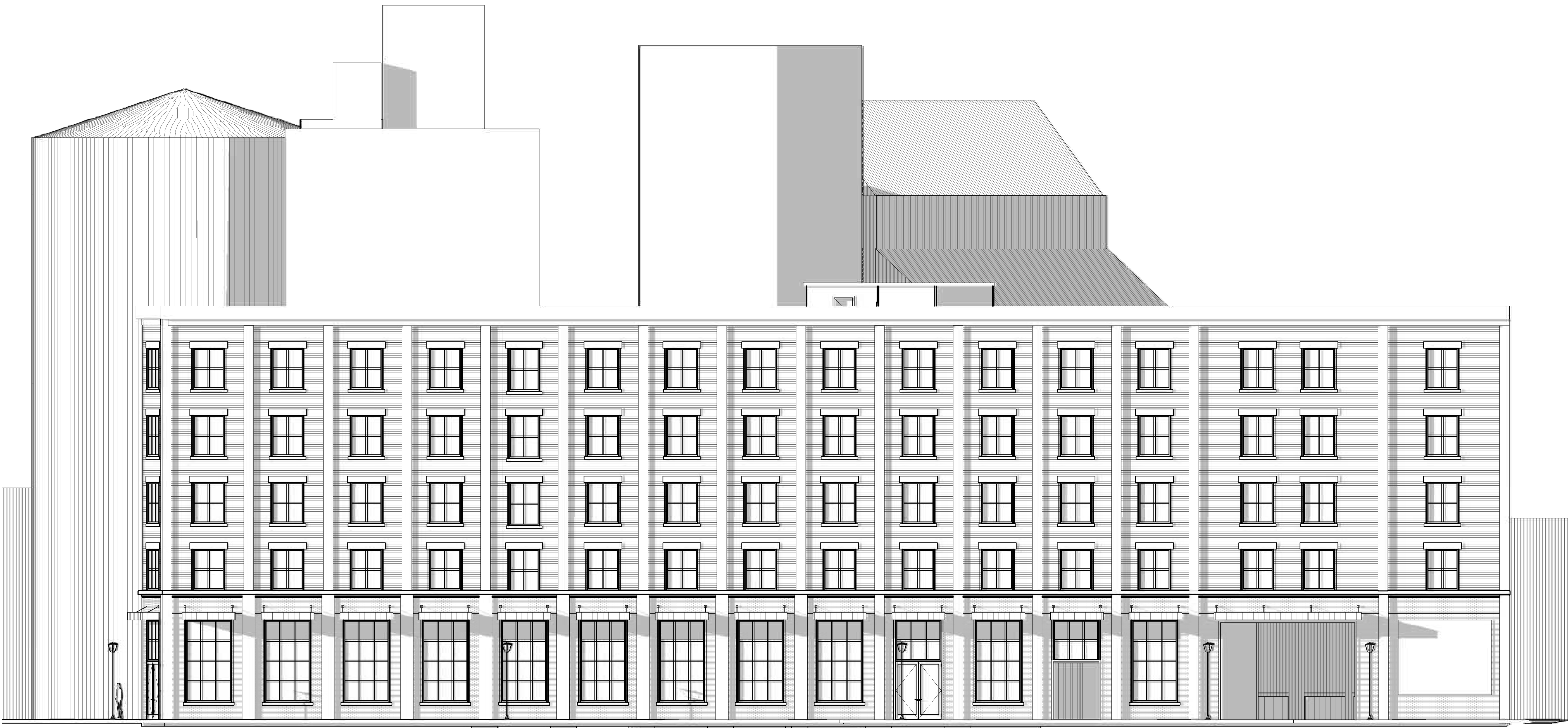
A5.3 North Elevation scale 1/8" = 1'
